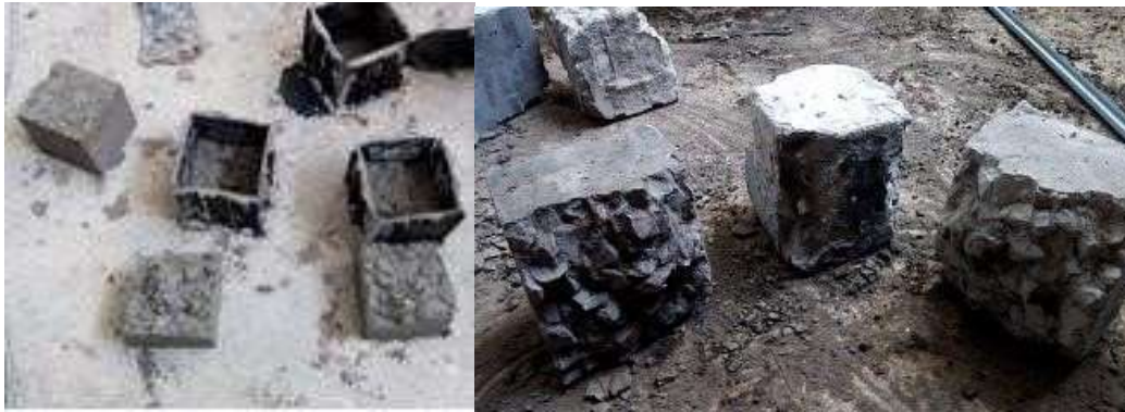
Fig. 8. Effect of substantial dosage of Lemon juice and Plastiment BV40
