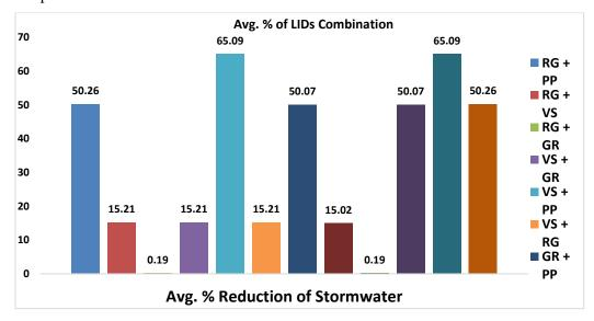
Fig. 9: Average percentage reduction of stormwater generation using varieties of LID combination.
