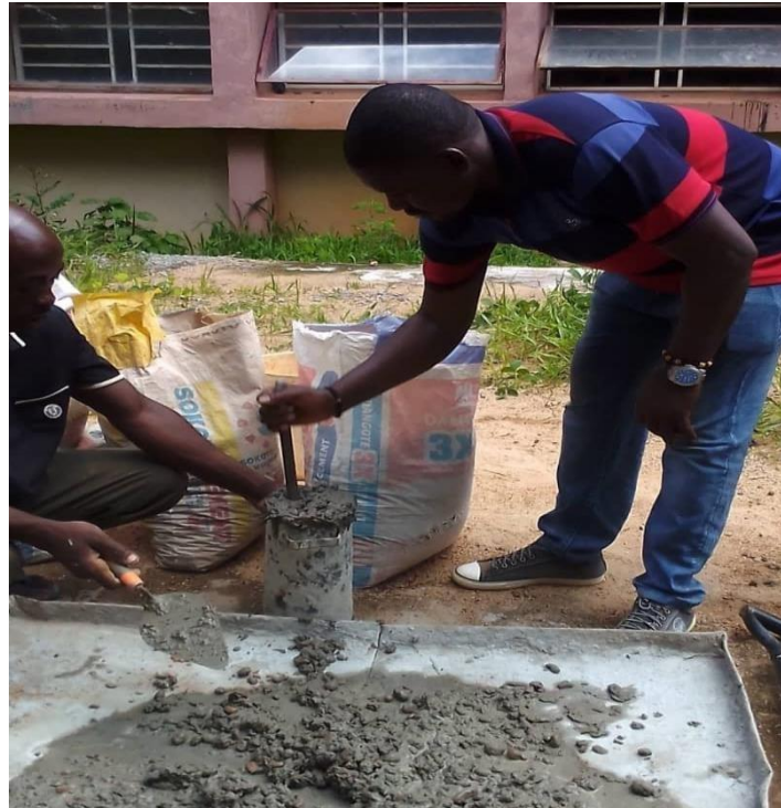
Fig. 3.: Fresh properties test in progress
