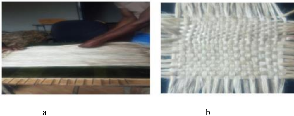
Fig. 2. Preparation of fiber orientation, a) Unilateral and b) Bilateral
