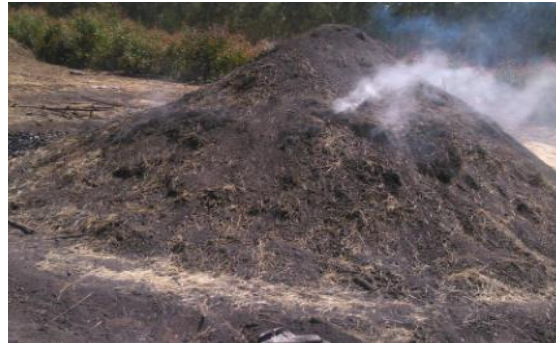
Fig. 1. Local charcoal making (earth mound kiln) and cover straw
