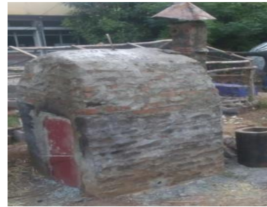
Fig. 3. (a) Model improved carbonization brick kiln. (b) Developed kiln
