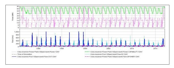
Figure 15. Power generated simulated for alternative 1 irrigation demand
