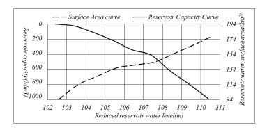
Figure.7. Forecasted Storage-Area Elevation Curve to 2015 from Sedimentation Surveys
