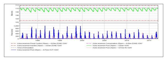
Figure 20. Reservoir water level for simulation of alternative 3 water demand
