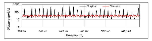
Figure 19. Reservoir outflow and monthly irrigation water demand for alternative 2
