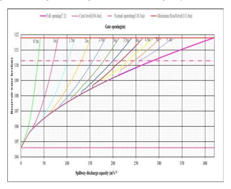
Figure 8. Spillway discharge capacity for different gate opening size
