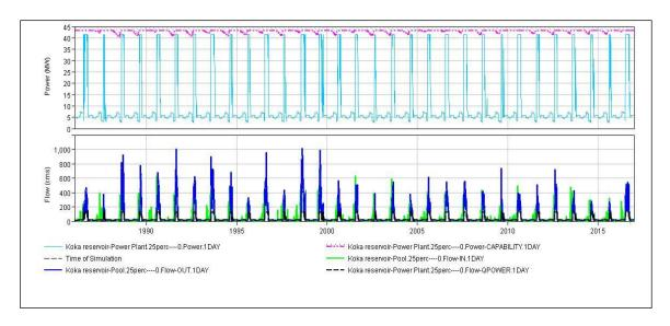
Figure 21. Power generated for simulation of alternative 3 water demand
