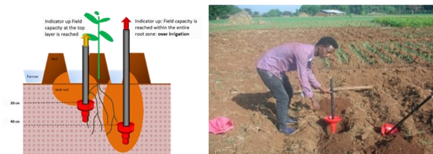
Figure 2: Schematic diagram for the installation of the wetting front detector according to Stirzaker et al. (2004) (left) with an example for onion (right).
