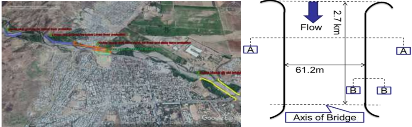
Figure 21: proposed Levee system of Kulfo River: The centre line representing the river, and the other two lines representing 25m offset to start the levee embankment (Left); Plan design of guide banks for upstream bridge)
