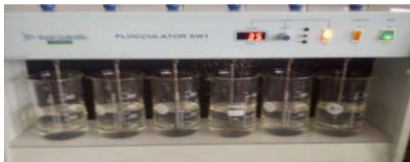
Figure 1: Experimental set up of coagulation for dose optimization
